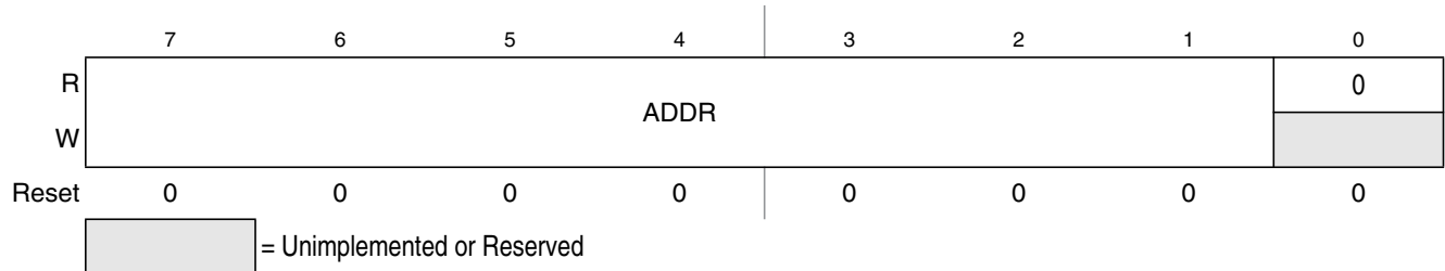
Figure 13-3. IIC Address Register (IIC1A)
